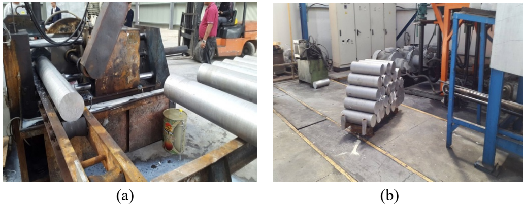
Figure 3. (a) cutting machine of the ingots, (b) ingots after the cutting process
